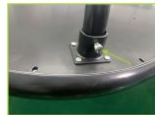
3. Use a M6*8 screw to secure a elbow pipe, a total of three elbow pipes.
