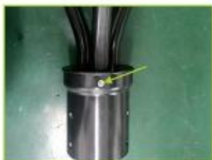
4. Fix the elbow pipes with three M6*12 screws.
